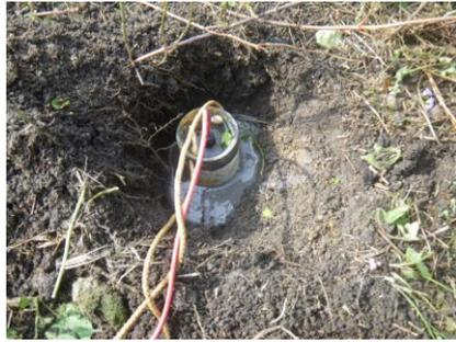
(c)電場量測之電極設置
